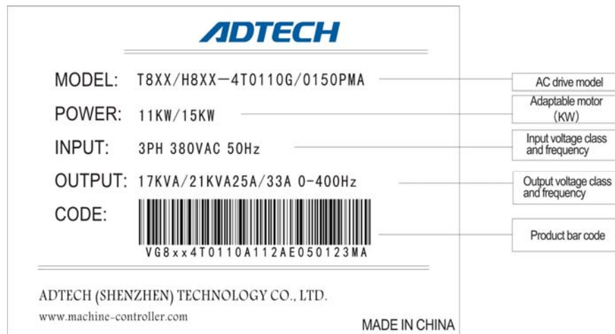
Figure 2-2 Description of T8 nameplate
